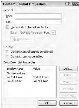
Figure 1-9: Click the Add button to create options for a drop-down list or combo box.
